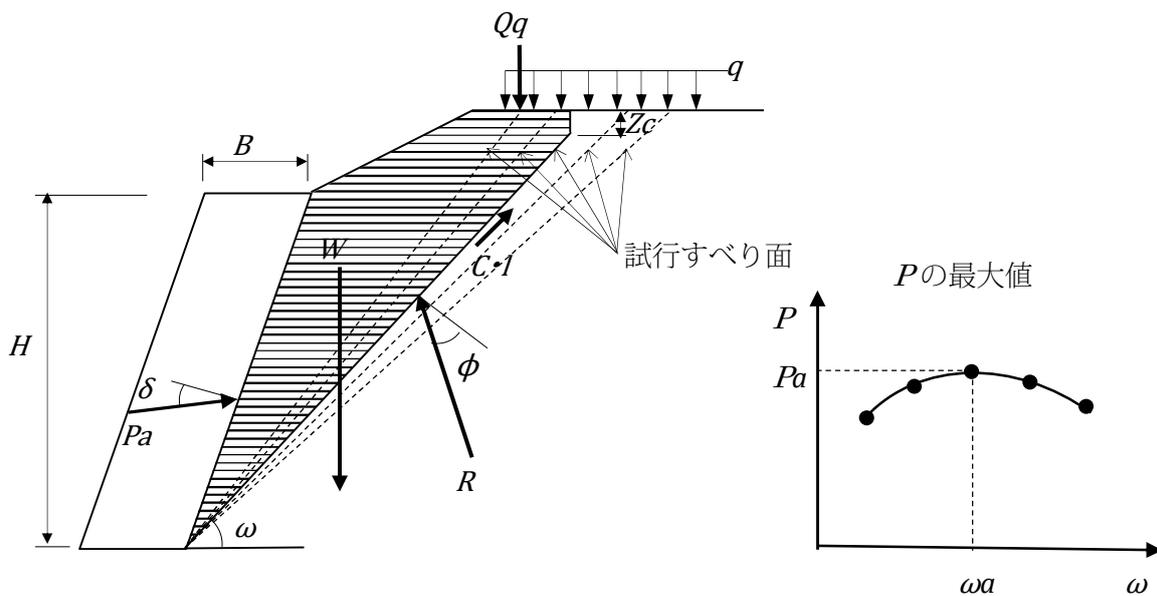
$$P = \frac{\sin(\omega - \phi)}{\cos(\omega - \phi - \delta - \alpha)} W$$
